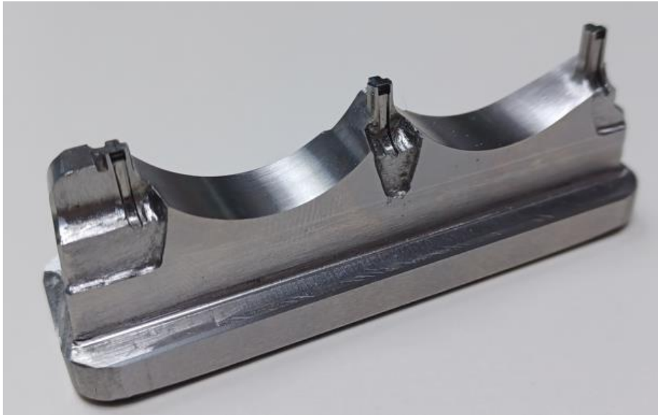
Figure FFF: Final geometry of the L-PBF insert, after finishing.
