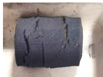
Figure 27: H13 samples after debinding with heating rate of 1 °C/min.
