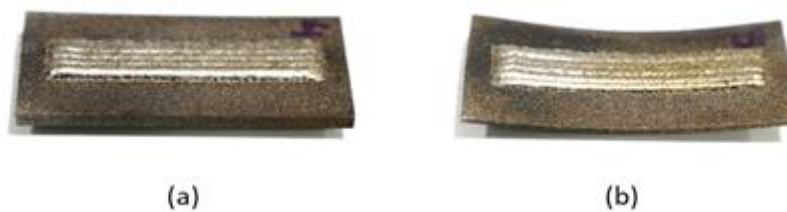
Figure 4: Samples 6 and 7 after deposition. The warpage observed is significant, especially on sample 7.
