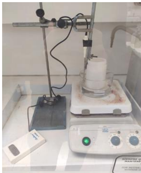
Figure 30: Laboratory set up for chemical debinding.
