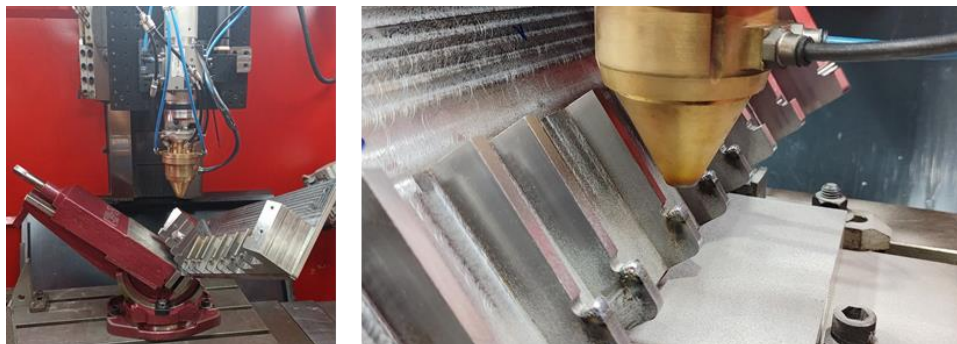
Figure 18: Demonstrator part fabrication setup in L-DED.
