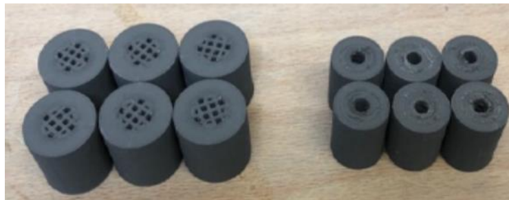
Figure 22: Samples for improving debinding and sintering
