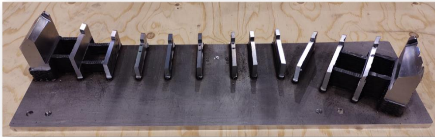
Figure 13. Machined critical zones of the demonstrator.
